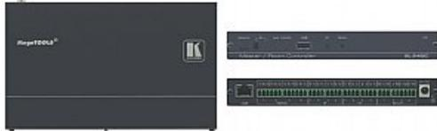
SL-240C is a compact master/space controller (Kramer Control brain) with PoE. It can operate over Ethernet with control interfaces that include: four bidirectional RS-232, four IR, four GPI/O, and four relays. It controls devices such as scalers, video displays, audio amplifiers, Blu-ray players, sensors, screens, shades, door locks, and lights. Multiple Kramer Ethernet control gateways can be used to add remote I/O ports
